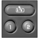
The controls for the memory function are located on the driver's door trim panel.
